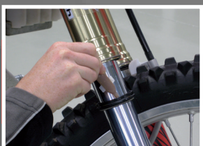
5. Apply grease on dust seal
